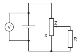
Which statement explains the change to the reading of the voltmeter as contact Z is moved towards end X of the potentiometer?
