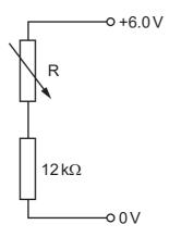
What is the resistance of the variable resistor R to give a potential difference of 1.0 V across the  $12 \, k\Omega$  resistor?
